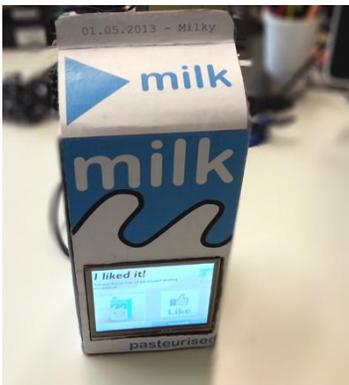
**Figure 3.** Pictures of the milk carton with the Gadgeteer touchscreen integration
